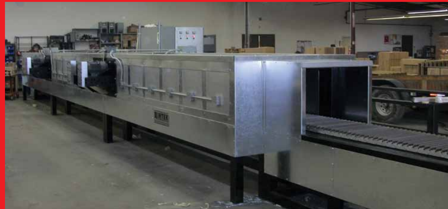
Large Custom Hybrid (IR/Convection) with Slat Conveyor
