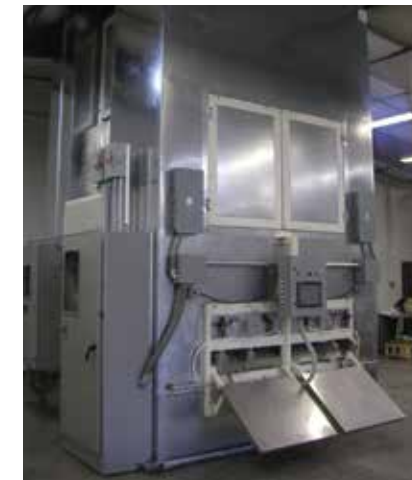
Ferris Wheel Vertical Conveyor
