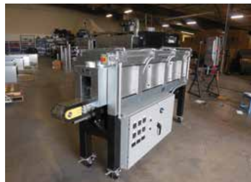
Small Oven with Slat Conveyor
