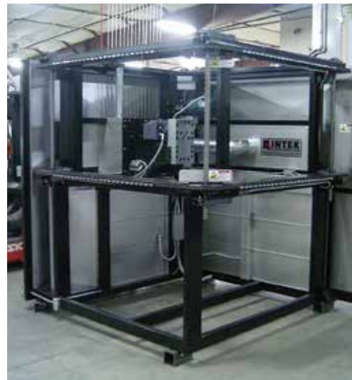
Horizontal Chain Driven Conveyor Oven
