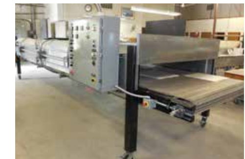
Multi-zoned Oven with Flat Wire on Edge Belt Conveyor
