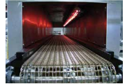
Gas Fired IR Tunnel
